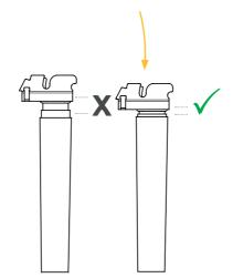
If the column extracts when turned upside down, turn the spindel clockwise until the end.
